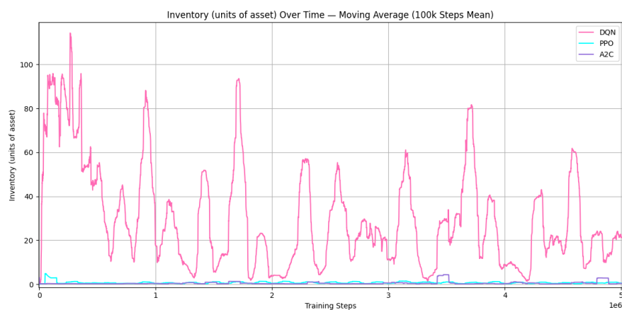
FIGURE 5.2: Inventory levels over time (compact state-action space setup with 4 observable states and 5 discrete actions)
