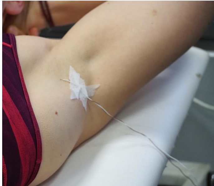
Figure 11. T- type thermocouple (RS Components), which measures temporal changes in local skin temperature.
