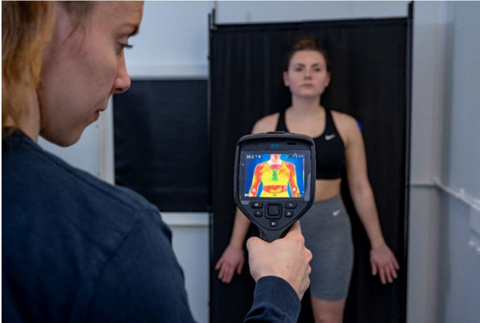
Figure 13. Handheld infrared thermography camera for thermal imagery of local skin temperature.
