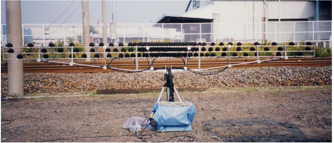
Figure 5.1 Microphone array in wayside horizontal position (MY13)
