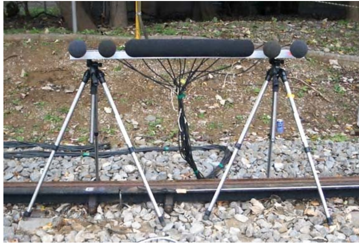
Figure 6.14 Microphone array used for the sound measurements
