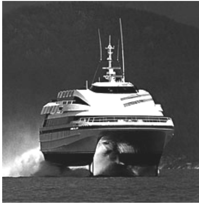
Figure D - 41: Example of a foil-catamaran, operating only on hydrofoil lift forces.
