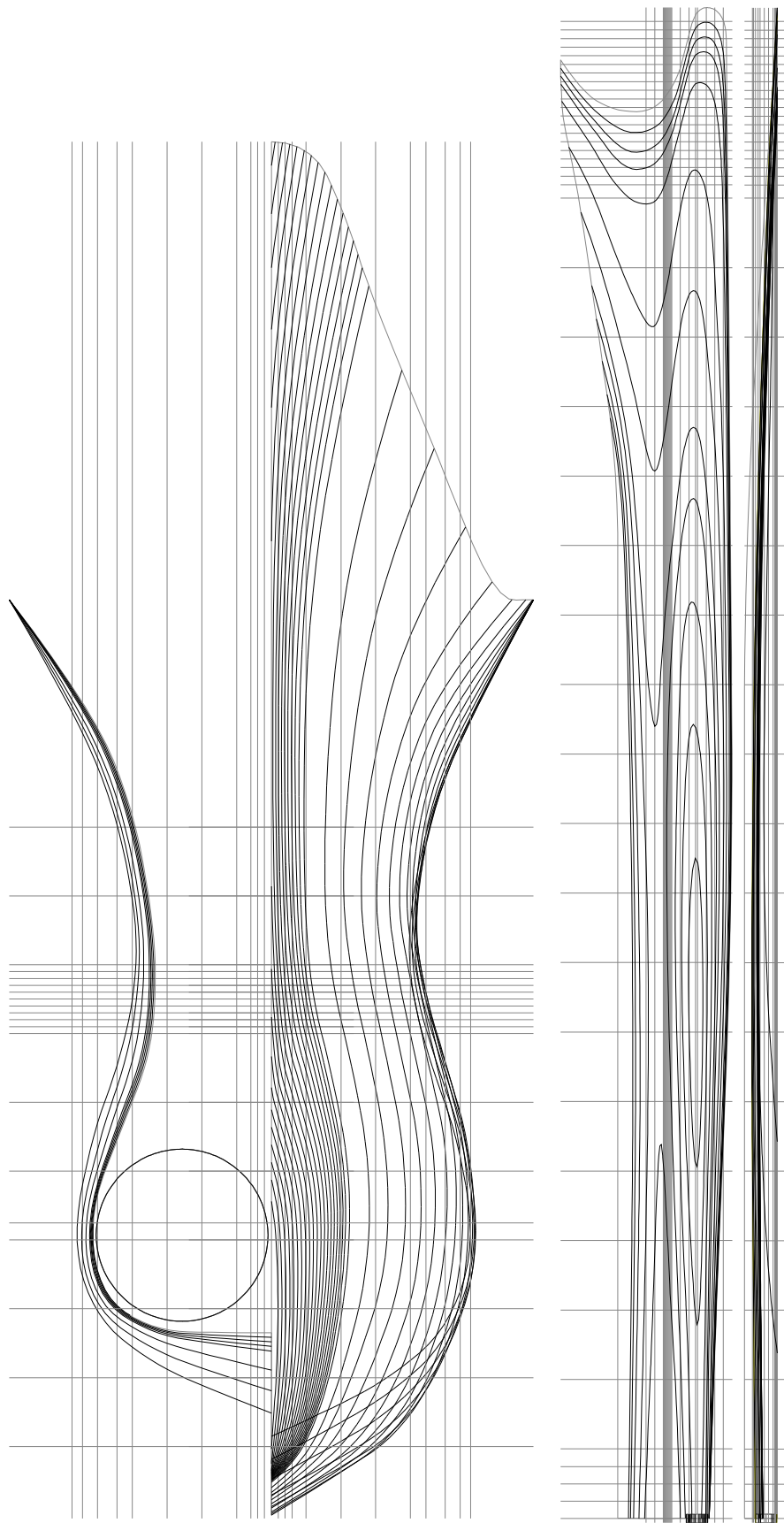
Figure 4.4: Linesplan of one demi-hull of the high-speed containership.
