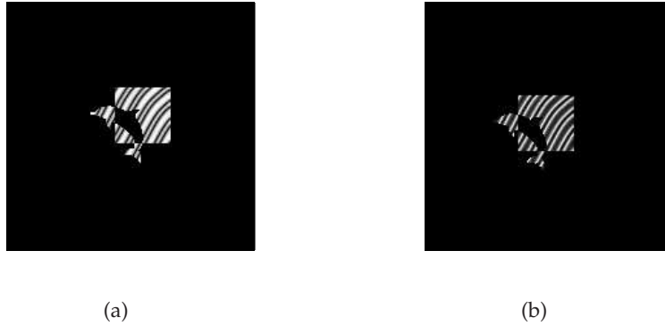
Figure 2.7: (a) The phase component of a complex valued object and (b) the reconstruction of this phase profile. Aside from the arbitrary phase shift which occurs, a perfect reconstruction of the phase profile is possible.
