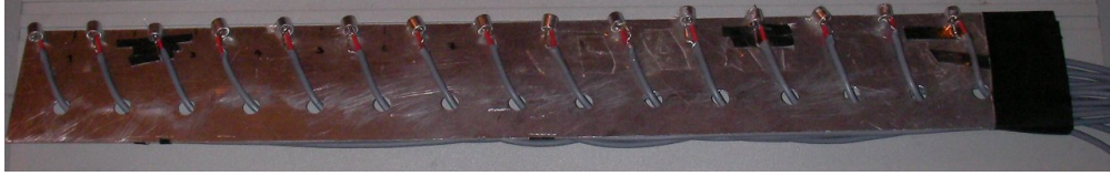
FIGURE 5.2: A photograph of the in-duct microphone array. Fifteen 7 mm electret microphones were mounted on a thin 50 mm by 400 mm aluminium plate. The microphones were positioned at the edge of the plate, with the centre of the capsules 25 mm apart.
