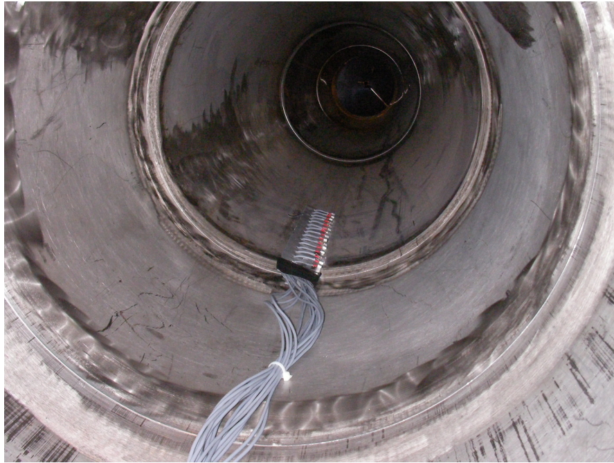
FIGURE 5.3: A photograph of the microphone array positioned in the duct. The microphones themselves lay on an axial line, and are as close as possible to the duct wall.
