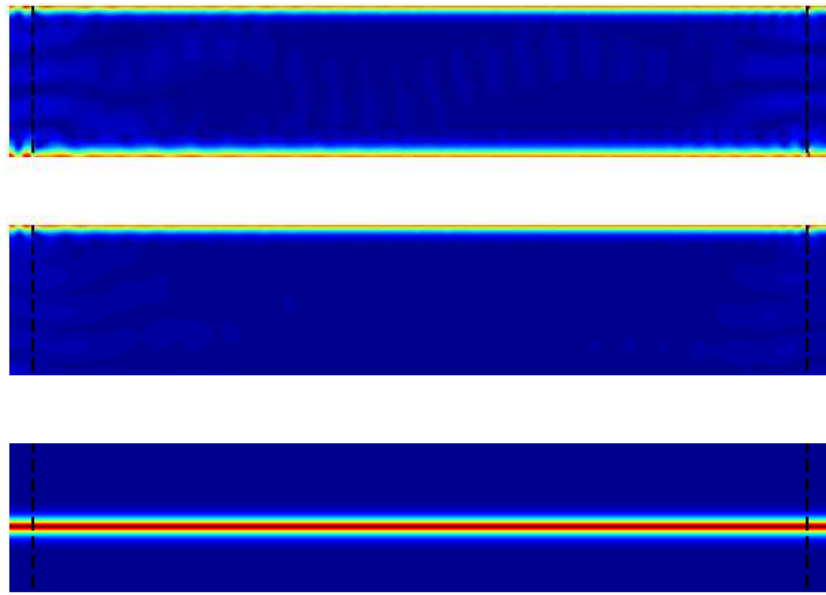
FIGURE 7.10: Pressure field contours due to vortical mode sources at k_0 = 30.94355 for a finite length lined duct with a linear sheared flow (negative gradient). Location of the leading and trailing edges of the liner is indicated by vertical dashed lines. Top plot, 2 incident vortical modes located at hub and casing ; Middle plot, single incident vortical mode located at casing; Bottom plot, single incident vortical mode located mid-duct. R = 1 , M_r = 0.012 , D = 0.021 , l_I = l_{III} = 0.067879 , l_{II} = 2.226446 , \bar{h} = 0.56897 .
