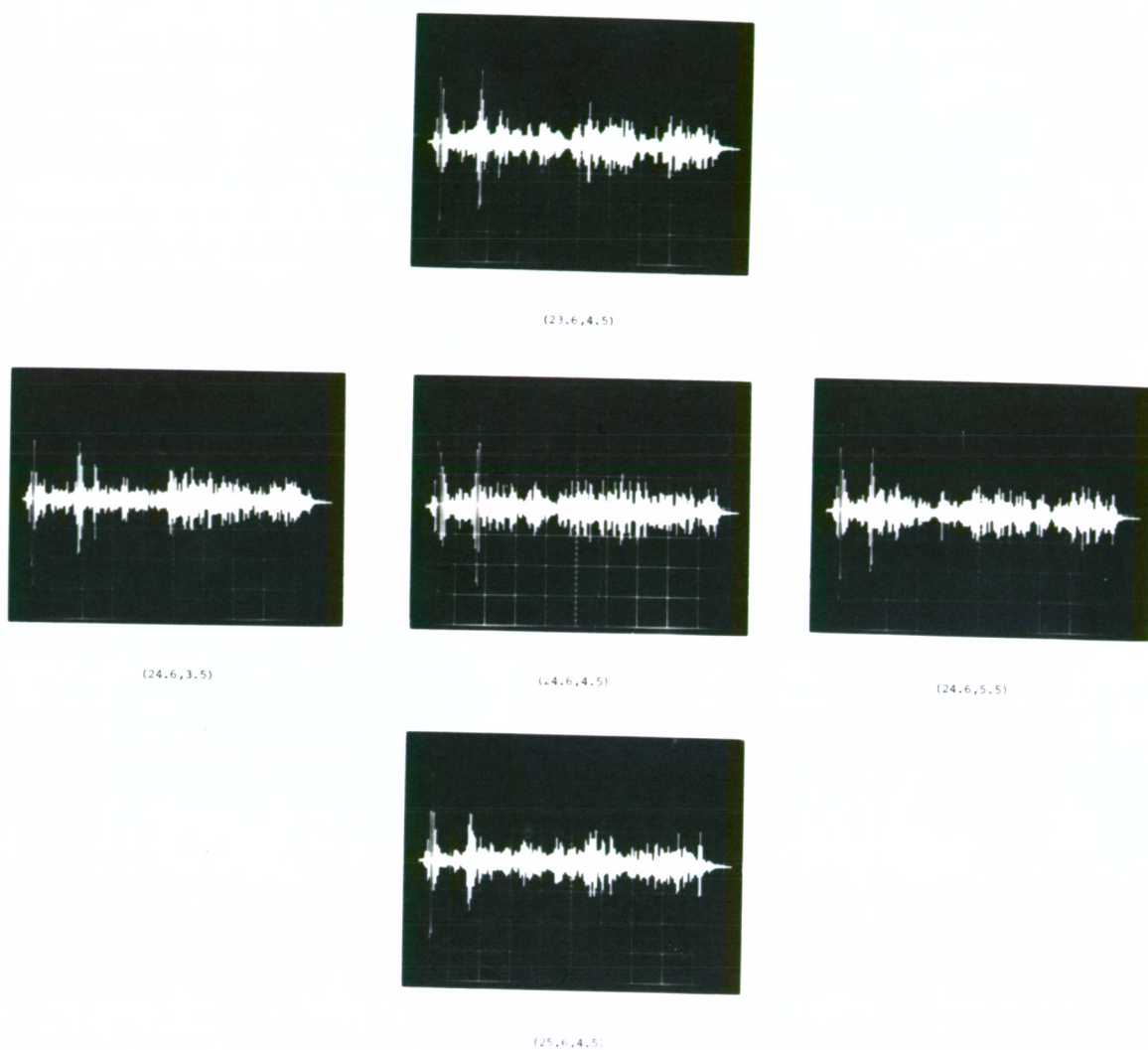
Figure 17.16. 2 kHz. oscillograms of 5 neighbouring receiver positions (receiver coordinates in m). 10 ms/div. sweep rate.
