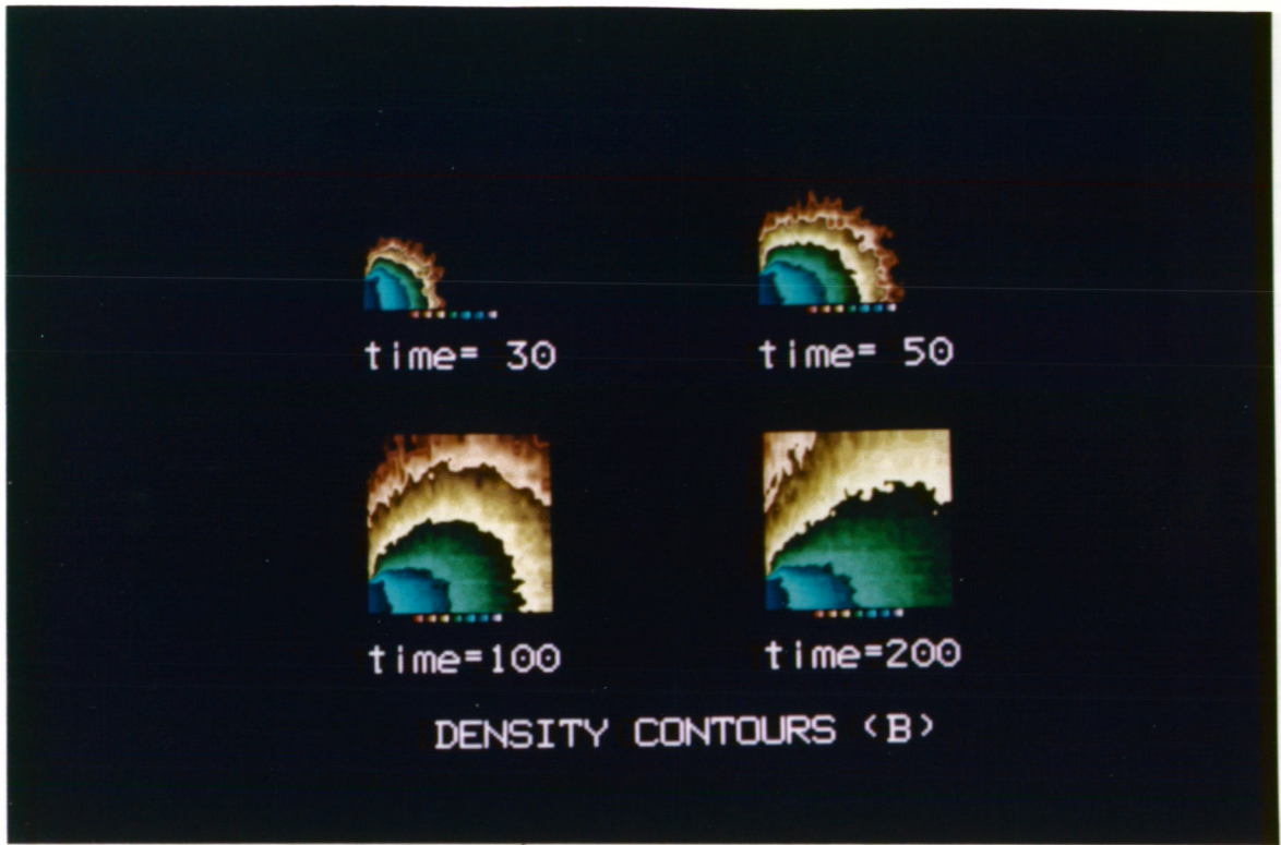
Fig. 4.29 Unsteady density contours at several time stations calculated with Bird's (B) Time Counter method.
