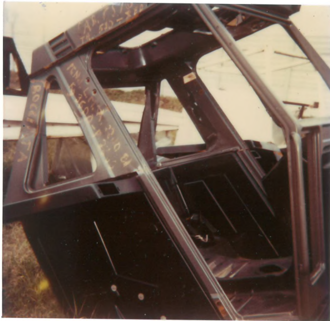
Figure 4.1 - Picture of the major parts of the safety cab: right side of the cover.
