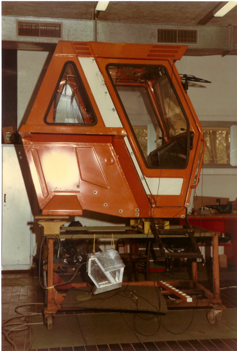
Figure 4.6 Rear supports attached to the lateral side panels.
