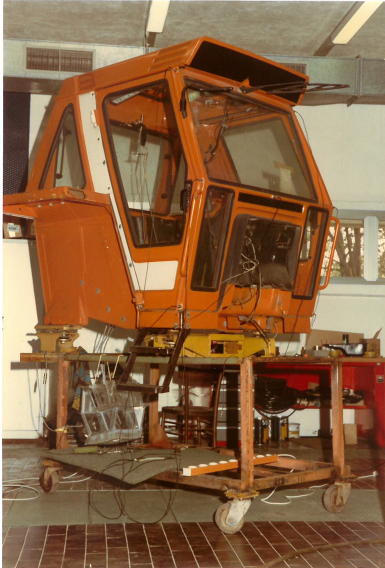
Figure 4.23 Picture of the whole cab mounted on a movable frame through four resilient supports.
