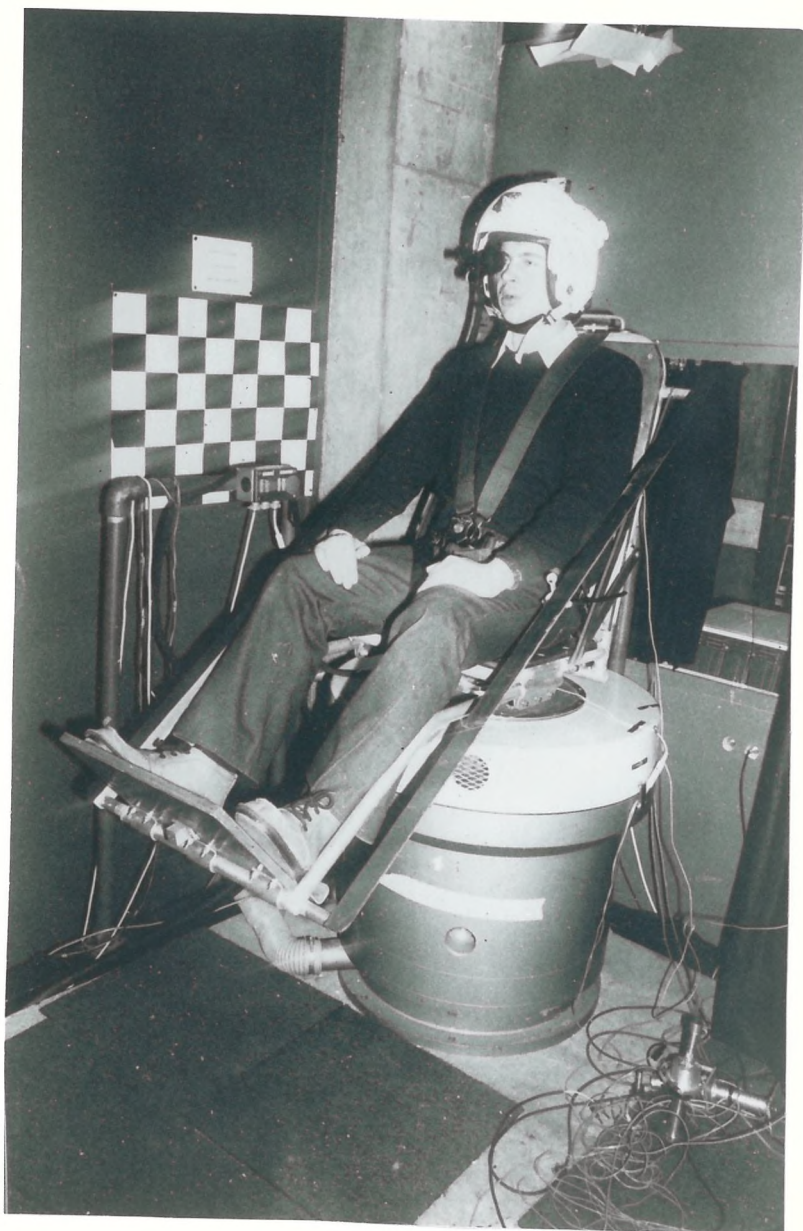
Figure 3.3.4. Subject Seated on Vibrator Wearing Restraint System and Helmet-Mounted Display
