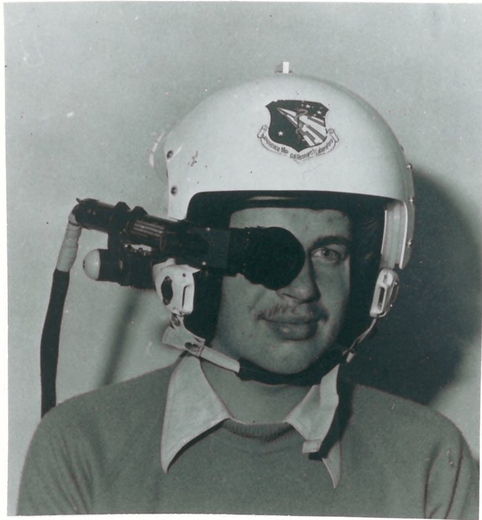
Figure 3.2.3. Subject Wearing Flight Helmet with Helmet-Mounted Display Unit Attached
