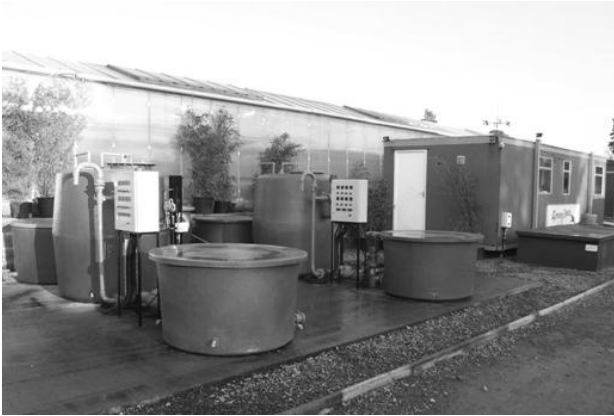
Plate 1. Pilot scale digesters used in the study
