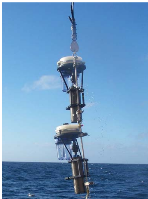
Figure II - 10: Example of two SAPS systems mounted on a stainless steel cable ready for deployment during D300. The top SAPS is for iron and trace metals analysis, the bottom SAPS is for POC/PON and ^{234}\text{Th} analysis.
