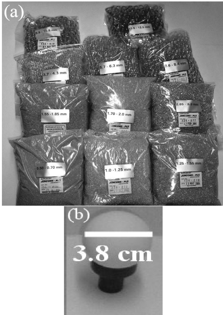
Figure 4.10: (a) Soda lime glass micro-spheres and (b) stone phantom.
