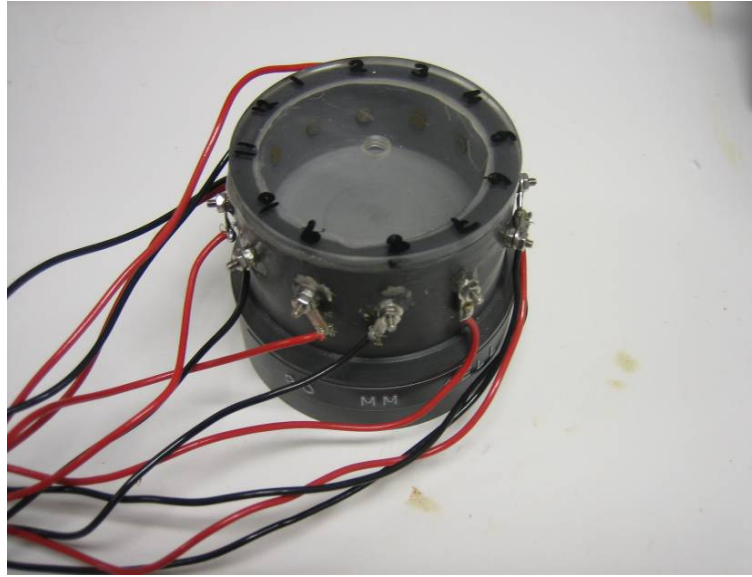
Figure 5.19 Electrical brine cell used to calculate the geometric factors for the sediment samples. The inside of the cell has the same dimensions of the sediment samples.
