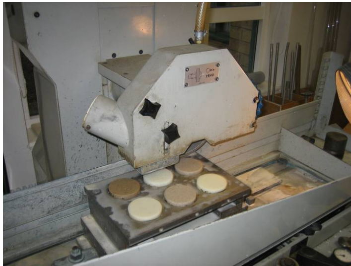
Figure 5.26 Synthetic sediment samples being ground down so that the sides of the samples were flat and parallel.
