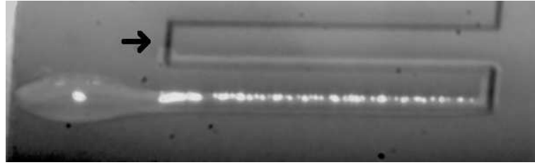
FIGURE 2.11: Screen capture from film of drop spreading on a scanned pattern with sharp corners. Arrow indicates point at which spreading stopped.
