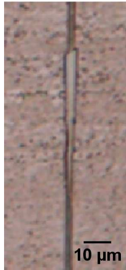
FIGURE 4.17: Optical microscope image of an inhibited domain formed at the end of a fast wall movement. Taper of inhibited domain illustrates deceleration of the domain wall.
