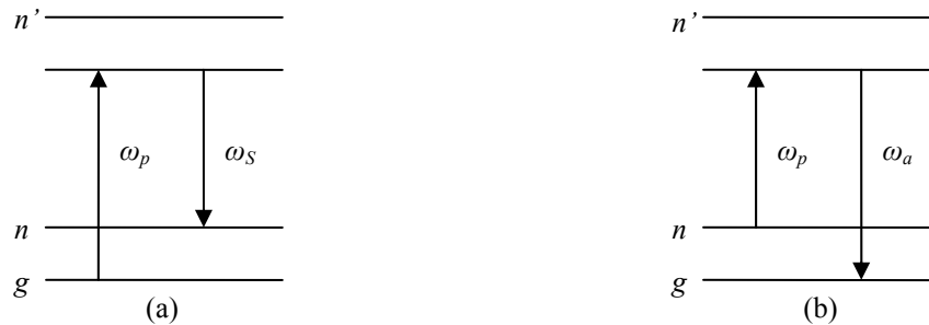
Fig. 2.5: Energy level diagram describing (a) Raman Stokes scattering and (b) Raman anti-Stokes scattering.
