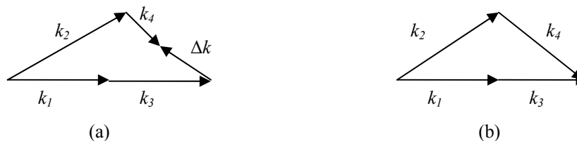
Fig. 2.7: A typical phase matching diagram where (a) a vector mismatch of \Delta k and (b) is the perfectly phase matched case (From [10]).
