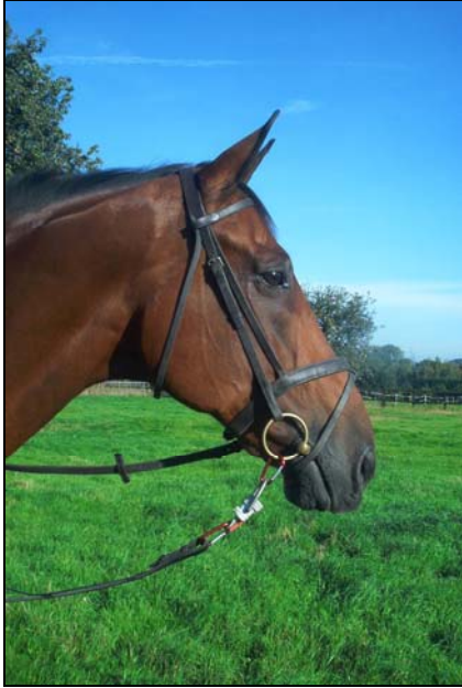
Figure 1. Force sensor fixed with clips between the snaffle and the rein.
