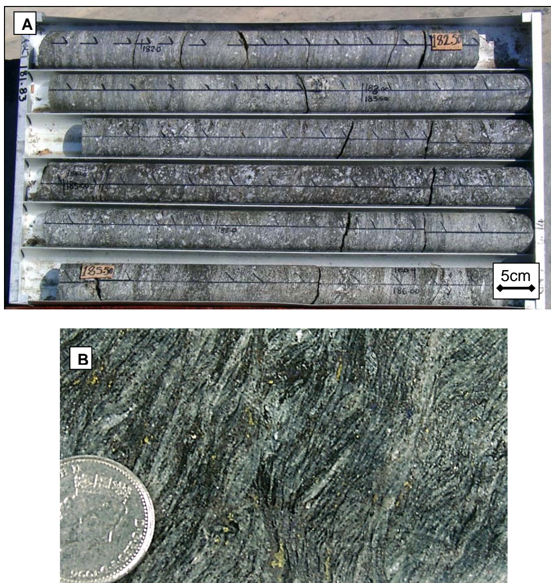
Figure 3.13 Photograph (COS - Eq-Chi-062) A) core tray of Chimiwungo ore schist with darker phlogopite rich zones and lighter zones dominated by muscovite B) Chimiwungo ore schist with asymmetrical extensional shearing developing sigmoid fabric
