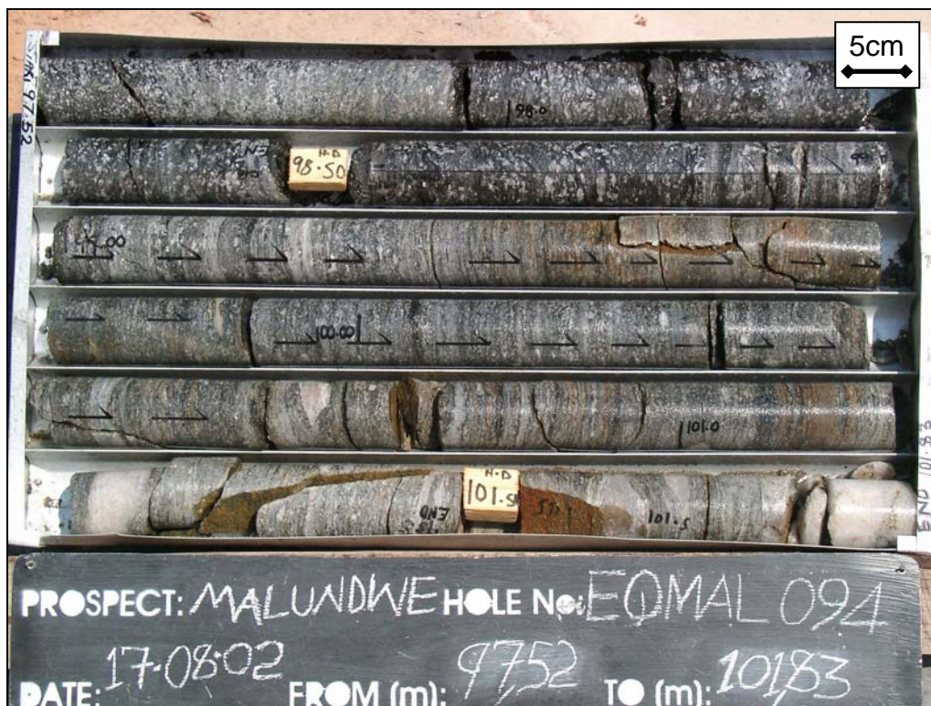
Figure 3.20 Photograph (Eq-Mal-094) Banded gneiss and mottled schist units from the Malundwe footwall
