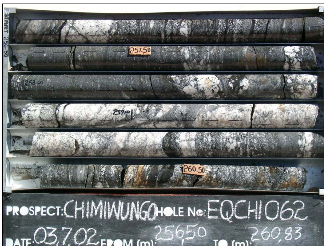
Figure 3.17 Photograph (Eq-Chi-062) Internal banded gneiss with amphibolite and internal quartz-feldspar pegmatite gneiss units
