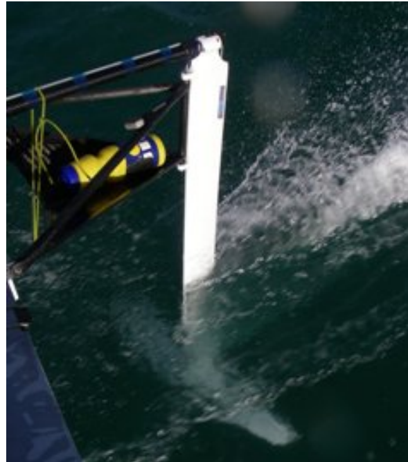
(b) Rudder mounted on gantry and showing lifting hydrofoil ('T-foil') at depth. Photo from [4]
