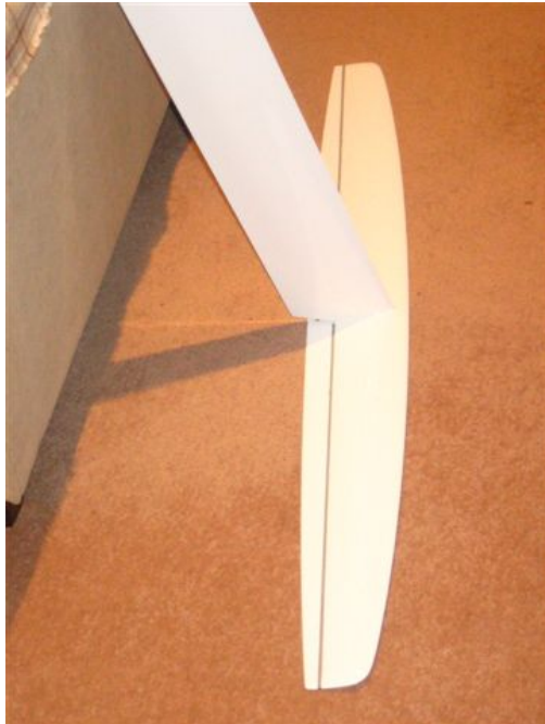
(a) Daggerboard and lifting hydrofoil ('T-foil'), showing trailing edge flap that is controlled by bow mounted wand sensor.
