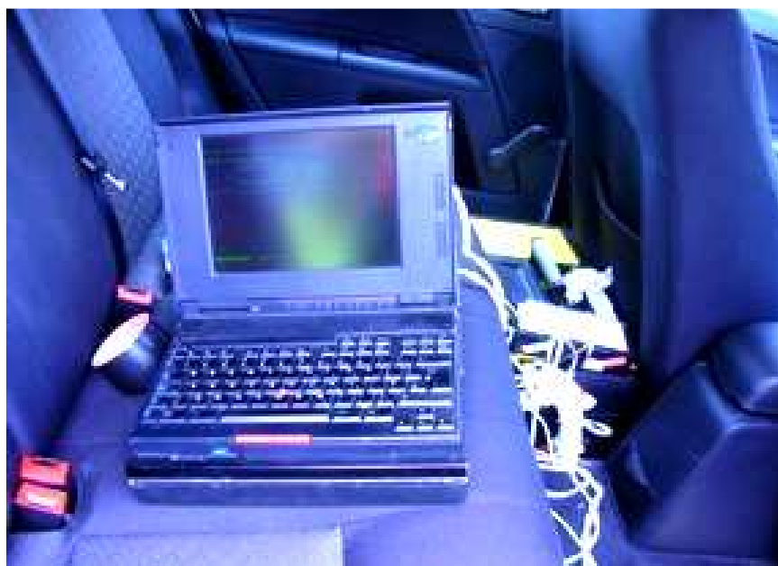
Figure 3.4. Measurement system (portable digital computer-based data acquisition and analysing system, HVLab (version 3.81) and 12-volt rechargeable battery
