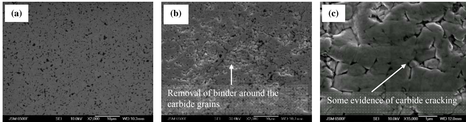
Figure 8.12: Comparison of sintered WC-5.7Co-0.3Cr sample; (a) unworn area, (b) pH 11 sample worn using 4.5 \mu\text{m} abrasives and (c) high magnification image of the worn sample showing preferential binder removal around the carbide grains (direction of abrasive motion: left to right).
