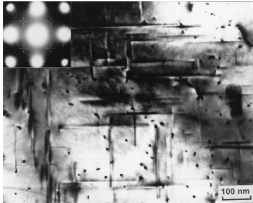
Figure 5.46 Precipitate morphology ( [001]_{\text{Al}} zone axis) of the sample of an AA6022 alloy heated to 300°C at 10°C/min immediately after solutionising and quenching. At this stage, rod-like and lath-like precipitates predominate (from reference [11])
