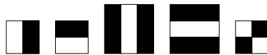
FIGURE 5.4: Illustration of the different kinds of features proposed by Viola and Jones. Each feature is the sum of the pixels values within the white regions subtracted from the sum of the pixels values within the black regions.
