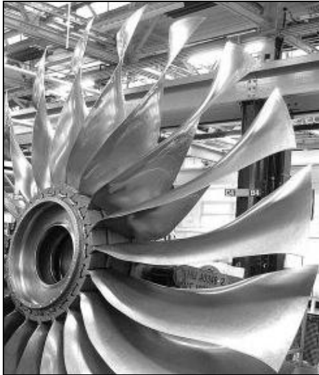
Figure 5: Traditional Rolls-Royce plc titanium fan blades.
