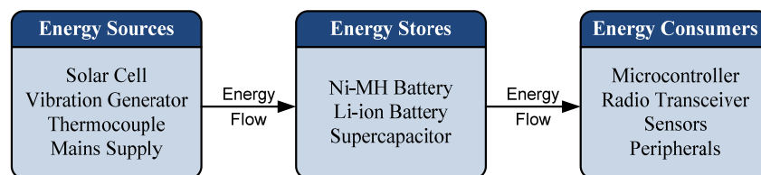
FIGURE 4-7 : The components of a node's energy subsystem, where energy is created by sources, is buffered by stores, following which it is used by consumers.
