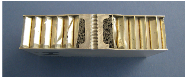
FIG 11. Image of a hot bonded reference sample sectioned after testing.
