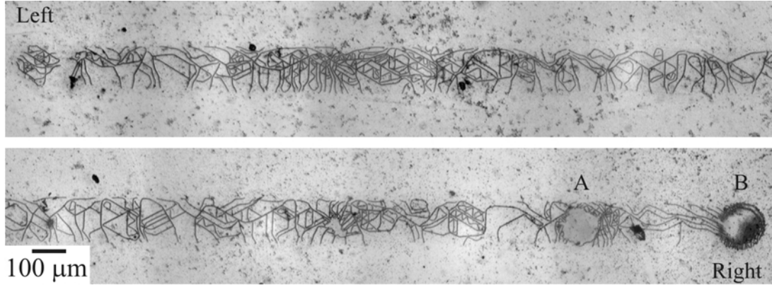
FIGURE 6.37: Self-organized lines following the fs-pulsed LAP scanning of \lambda = 400 nm light of I \simeq 4 GW/cm 2 , with E = 18 kV/mm bias in undoped CLN. Shown is a single continuous line of exposure where the right side of the top image connects to the left side of the bottom image.
