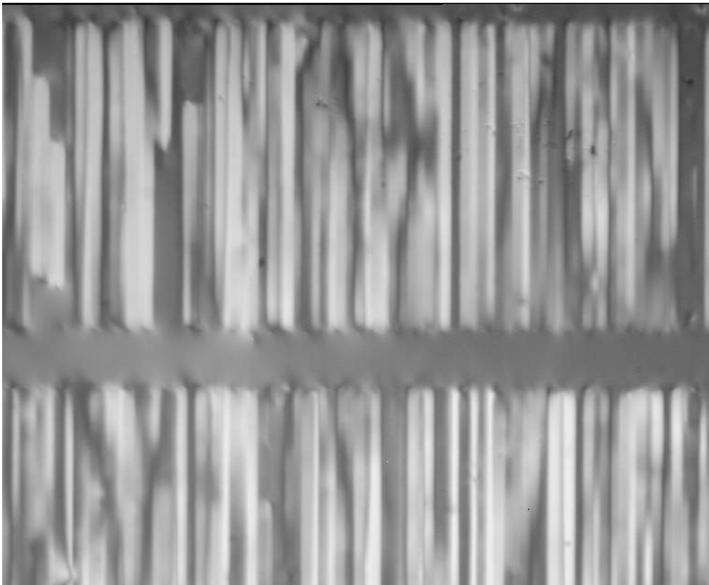
Figure 4.06. PPLN structure showing grating domain under a microscope using crossed polarizers.
