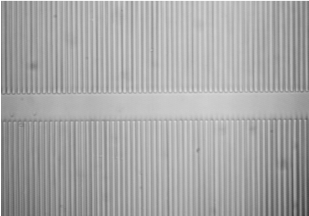
Figure 4.20. PPLN sample (code No.910) with 10μm period grating poled by gel electrode, the thickness of the photo-resist S1813 was 1.8μm. The uniformity of the grating is very good.
