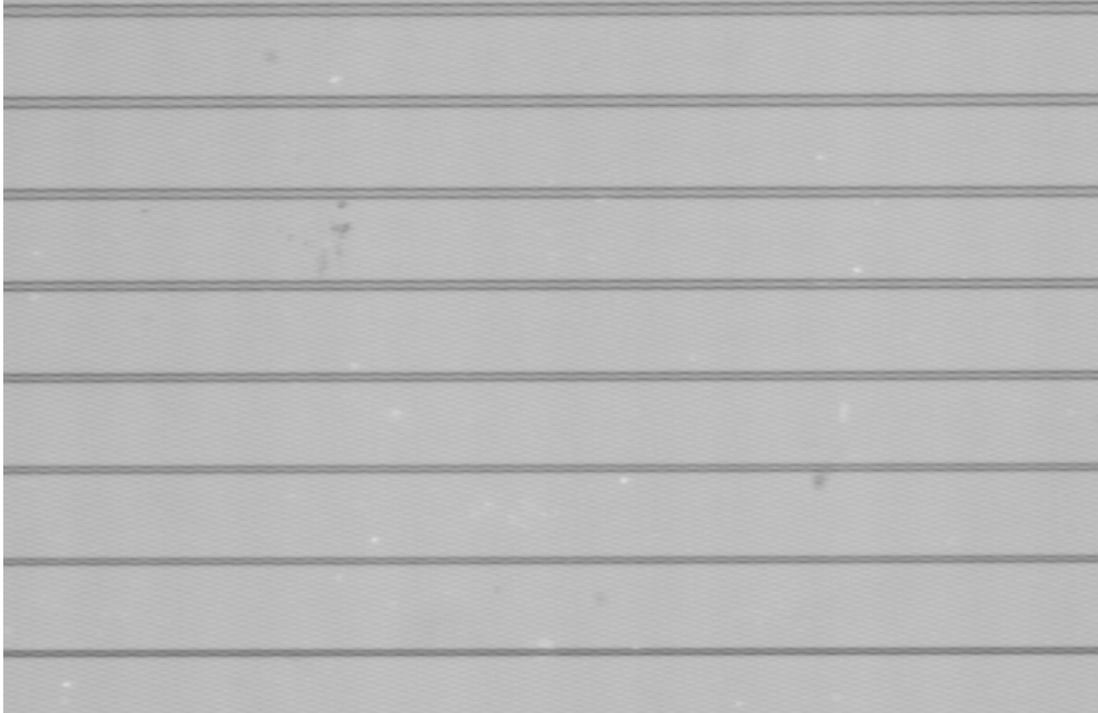
Figure 6.05. Patterning of the sample viewed under the microscope, the waveguide strips are spaced by 100 \mu m apart and are oriented parallel to the x -direction, with widths varying from 1.5 \mu m to 10 \mu m.
