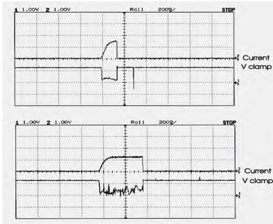
Figure 4.05. The current and voltage trace of poling processes, the upper plot shows the recorded trace for Q = 20\mu\text{C} , The bottom one shows trace for Q = 110\mu\text{C} .
