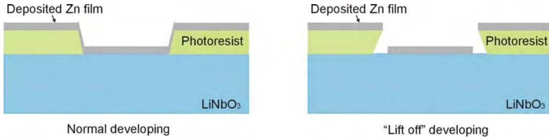
Figure 6.04. Schematic drawings of normal developing and "lift off" developing.
