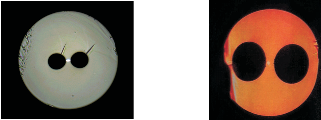
FIGURE 6.3: Images of twin-hole fibres fabricated in the in-house facilities of the ORC. (Left) ORC-1 fibre. (Right) ORC-2 fibre
