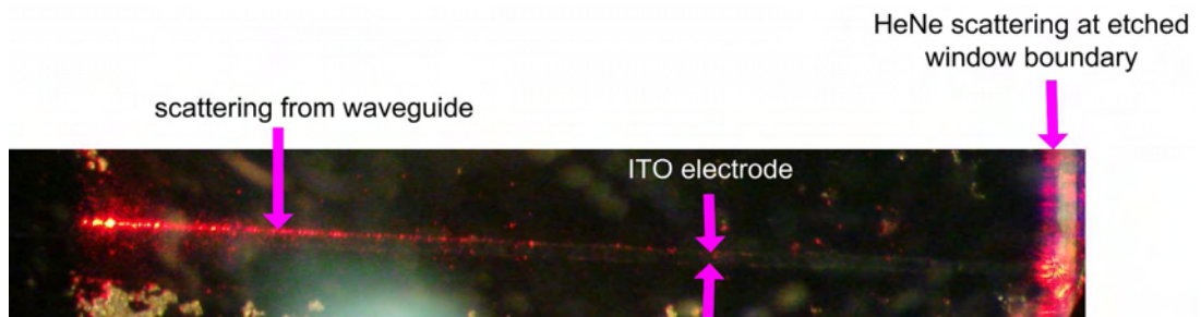
Figure 8.15 HeNe scattering from the waveguide showing non-optimised electrode position (offset).
