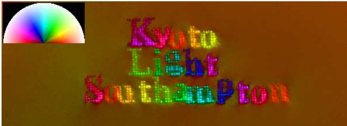
Figure 9.1: Type-II modification induced in fused silica by femtosecond laser direct writing. The different colour of each letter is corresponding to the different orientation of the slow axis of the birefringence.
