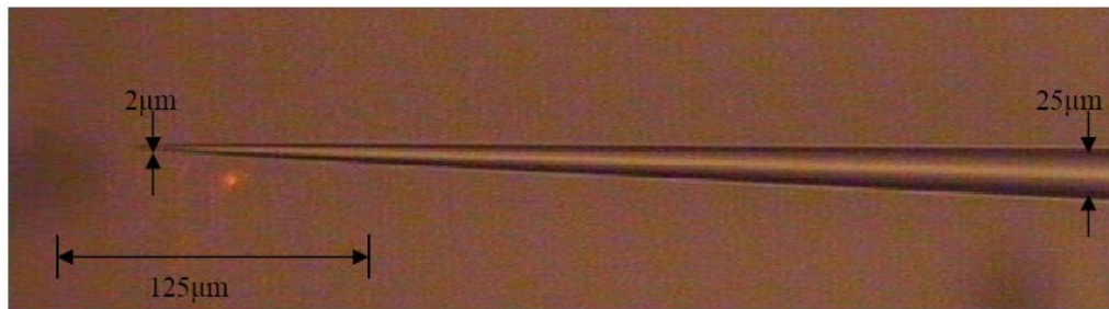
Fig. 2.9: Picture of a tapered fibre tip by P-2000.
