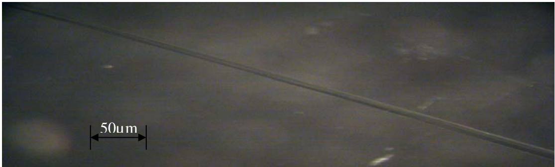
Fig. 2.6: Picture of a tapered fibre from the standard single mode fibre.
