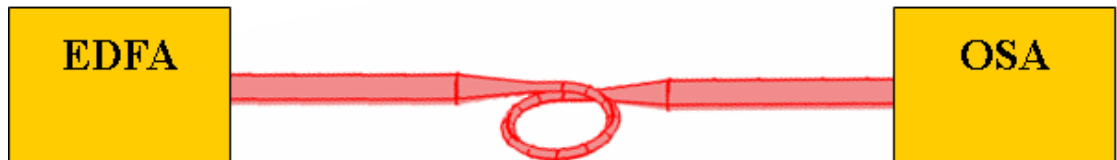
Fig. 6.5: Illustration of the spectrum measurement of an ONLR.
