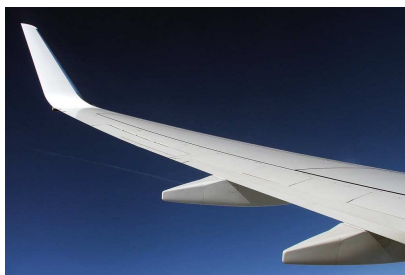
Figure 5-4 Example of a blended winglet on the Boeing 737-800.
