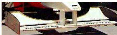
Figure 5-2 A racing car front wing, featuring end plates.
