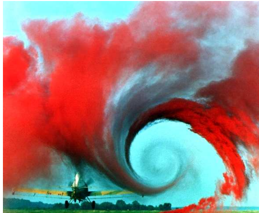
Figure 5-1 An aircraft wake vortex study performed by NASA.
