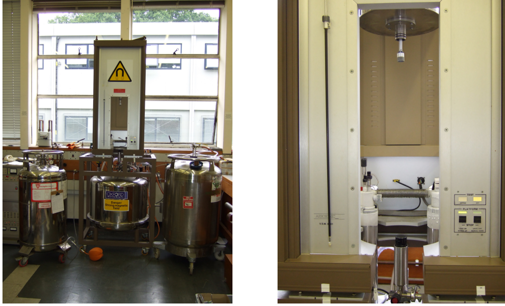
Figure 7.1: Vibrating sample magnetometer (VSM): the left photo of the complete set-up shows the actual VSM in the middle, with the transducer unit on the top and the cryostat vessel underneath. Adjacent are the helium containers required for the cooling of the cryostat. On the right photo, the vibration rod with the protruding sample holder can be seen on the top. On the bottom, the cryostat tail is visible that houses the sample holder during operation. The superconducting magnet has been removed.
