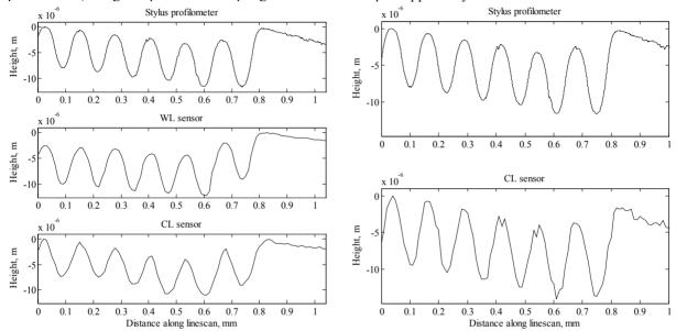
Fig. 1 (a) Groove cross-sections (cylinder reference #1) as measured by stylus profilometer (top axis), WL sensor (middle axis) and CL sensor (bottom axis). (b) Groove cross-sections as measured by stylus profilometer (top axis) and higher-resolution CL sensor (bottom axis). Scanning system samples at 10μm resolution along the linescan axis using both optical sensors, and at 0.25μm for the stylus profilometer.
