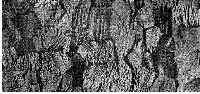
Figure 2.1: Bitter technique of magnetic powder used to show domain boundaries (reproduction from [6]).
