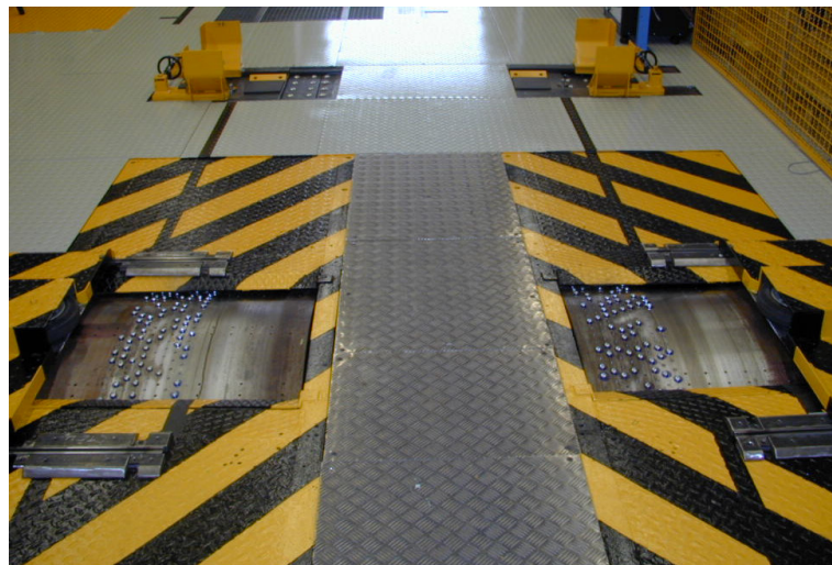
Figure 3-22 Vehicle road noise dynamometer with patented surface.
