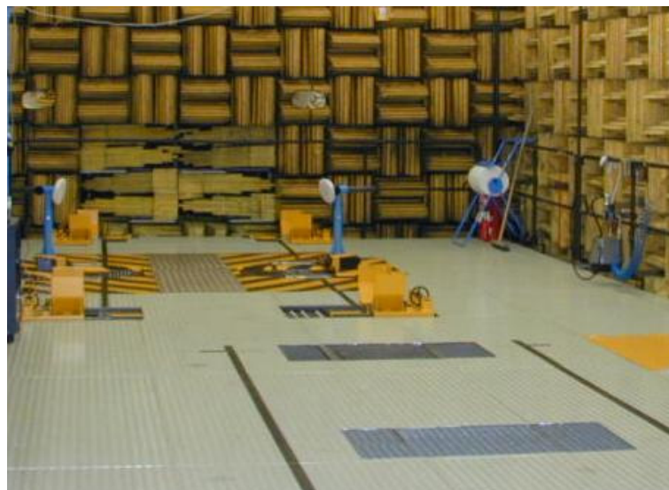
Figure 3-1 Semi-anechoic vehicle test chamber.
