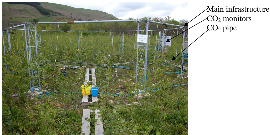
Figure 4.2.2. One of the FACE rings at the BangorFACE site. The CO 2 is released from pipes around the middle of the main infrastructure. Each ring has a CO 2 monitoring system.
