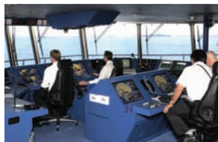
The integrated navigation system on the Superstar Virgo features 3 ECDIS
