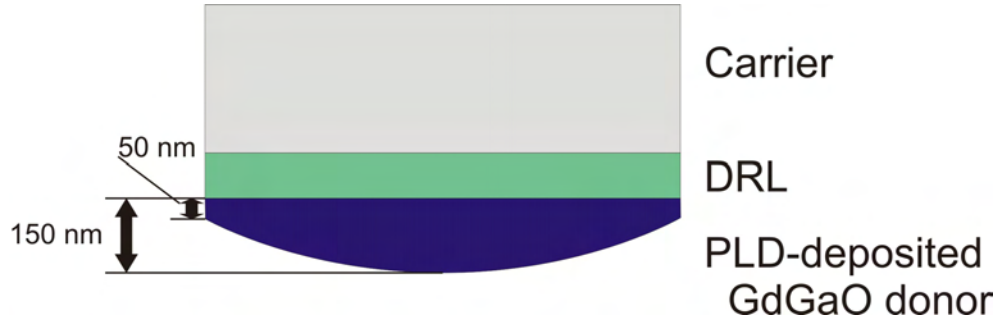
FIGURE 5.8: Schematic of how the thickness of the PLD-deposited GdGaO donor varied across the carrier.
