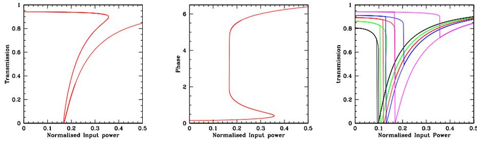
Fig. 3. Nonlinear response of a 3 turn microcoil resonator. Fig. (a) shows the full solution (both stable and unstable branches) as a function of the input power. Fig. (b) shows the output phase while Fig. (c) shows the hysteresis curves for the resonator for a range of wavelengths.
