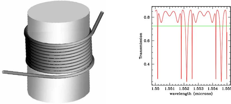
Fig. 1. (a) Schematic of a microcoil resonator taken from [2]. (b) Transmission spectrum for a lossy OMR with 8 coils. The loss is 0.02dB/mm while the coupling strength was  $3\text{mm}^{-1}$ . The green line shows the expected transmission for a straight length of fibre with the same length and loss.
