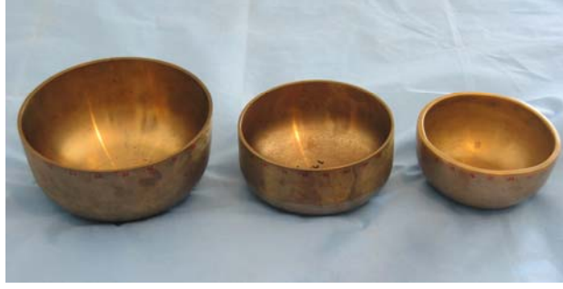
Figure 5.1. Three singing bowls used in the experiments: Bowl 1 ( \phi = 180 mm); Bowl 2 ( \phi = 152 mm); Bowl 3 ( \phi = 140 mm).
