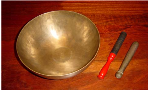
Figure 5.2. Large singing bowl: Bowl 4 ( \phi = 262 mm), and two pujas used in the experiments.
