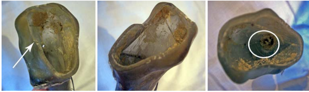
Figure 6-6 Femoral sawbone post modification. Adapted to best represent revision femora with widening of the internal medullary canal (circle) and thinning of the outer cortices (arrow).
