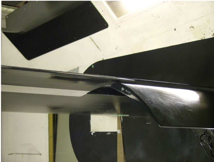
FIGURE 6.1: Picture of wind tunnel model with a split flap. Flow is from left to right.
