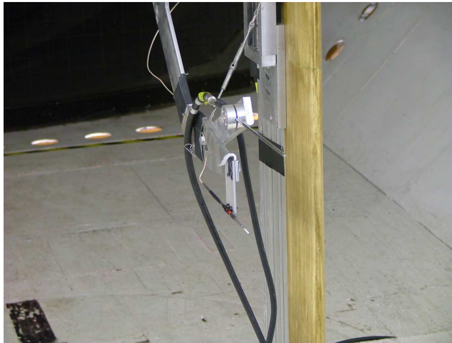
FIGURE 3.8: A view of the hotwire setup mounted on the one-dimensional traverse. The pitot-static tube is located above the hotwire probe and was used for calibration. View looking downstream.
