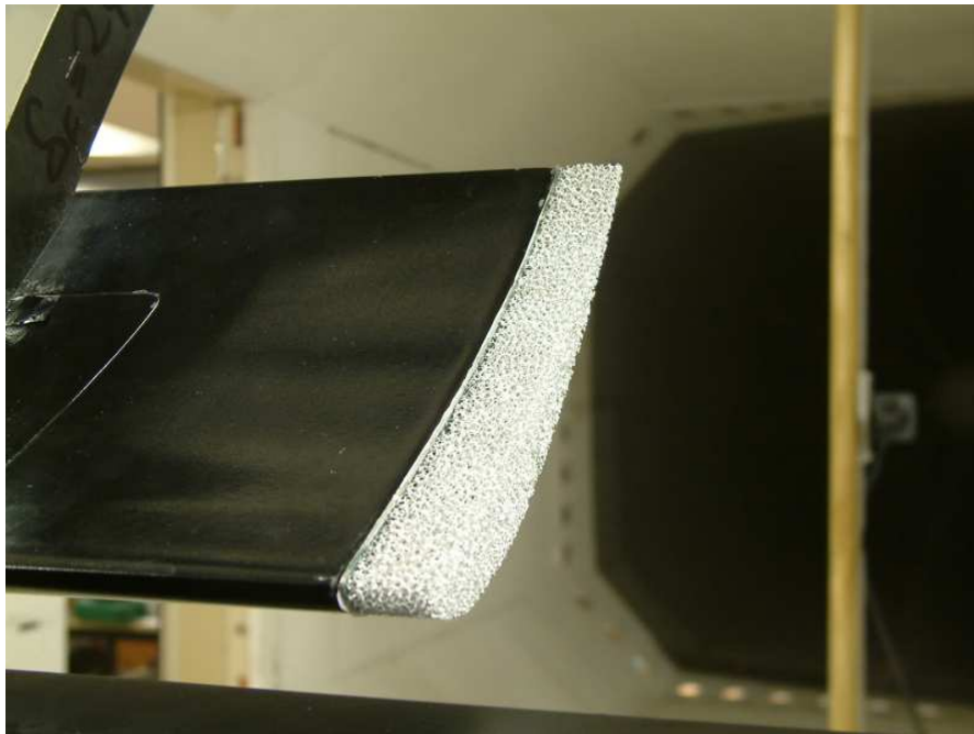
FIGURE 3.6: A downstream view of the porous flap side-edge. The PIV camera can be seen mounted on the strut in the background. The laser sheet shines from right to left in a vertical plane.
