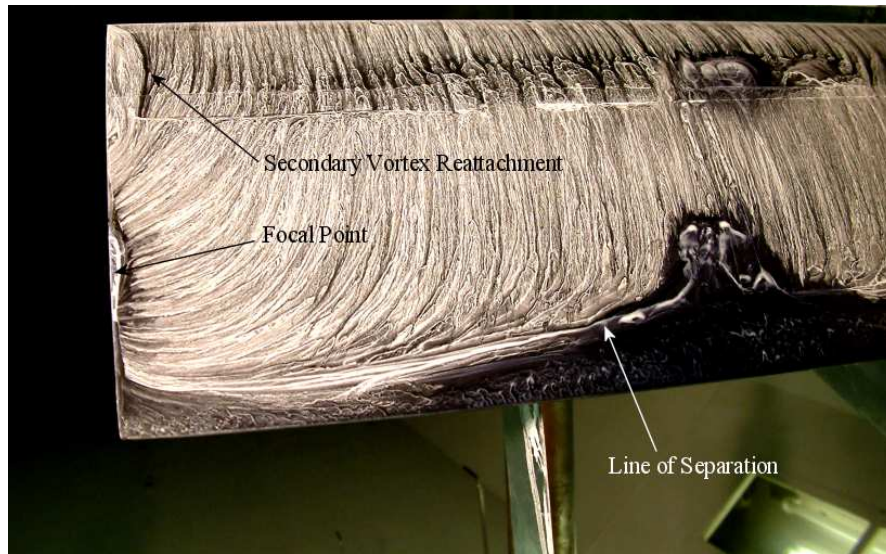
FIGURE 4.7: Oil flow of suction surface of flap. View looking upstream. V_\infty = 20 m/s.
