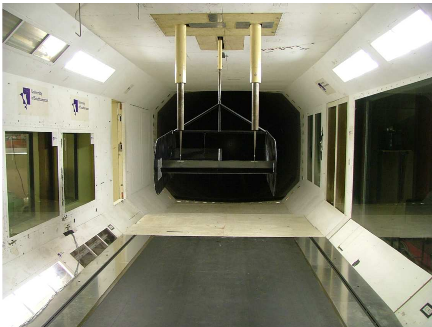
FIGURE 3.4: The wind tunnel model in-situ in the R.J. Mitchell wind tunnel.
