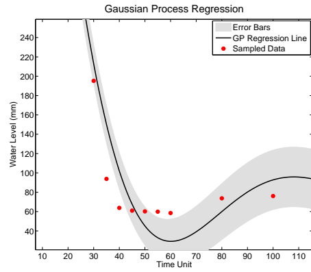
(b) Regression on sampled data taken between time unit 30 and 115, with 9 samples. FLOODNET node 1 collects Fisher information value of FI = 0.40650 \cdot 10^{-1} .
