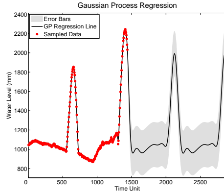
(d) GP regression on FLOODNET node 2 using a covariance function with period terms such that C = C_{sqe} + C_{per} + C_{noi} .
