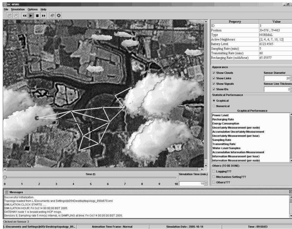
FIGURE 3.10: FLOODNET’s nodes sample from the environment.
