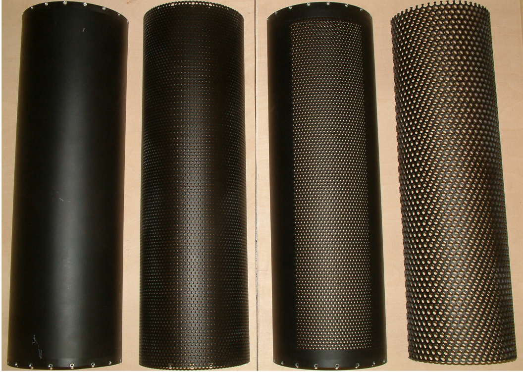
FIGURE 3.3: Picture of the 4 different shells subject to experiments, from left to right: solid, perf33, perf42 and perf55.
