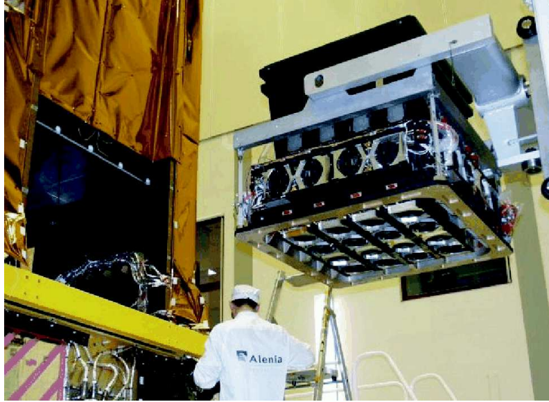
Figure 2.3: IBIS during the last phases of mechanical integration at ESTEC (Ubertini et al. 2003).
