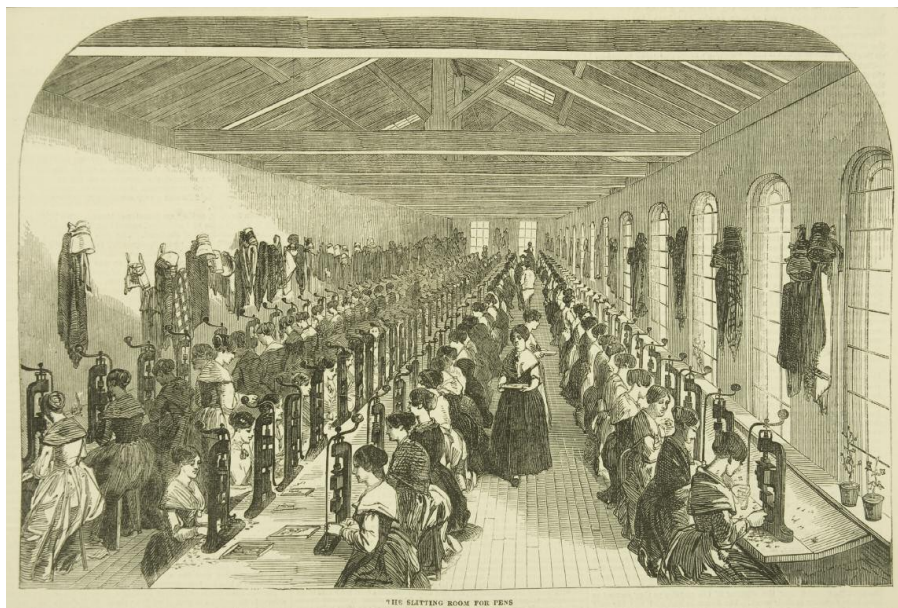
Plate 7 The slitting room for steel-nibbed pens in the factory of Messrs Hinks, Wells and Co., Birmingham, in 1851. The price of pen nibs was 6d. a gross in that year; in 1830 it had been 8s. Women were employed for their dexterity, and they have arrived well-dressed for work, with the pot plants on the window sill adding a homely touch. [ Illustrated London News , 1851 (part 1, p. 149)]
