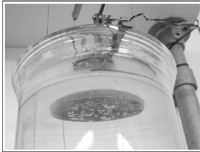
Fig. 5.6: Air bubbles forming on the settling column rough plate after deployment
